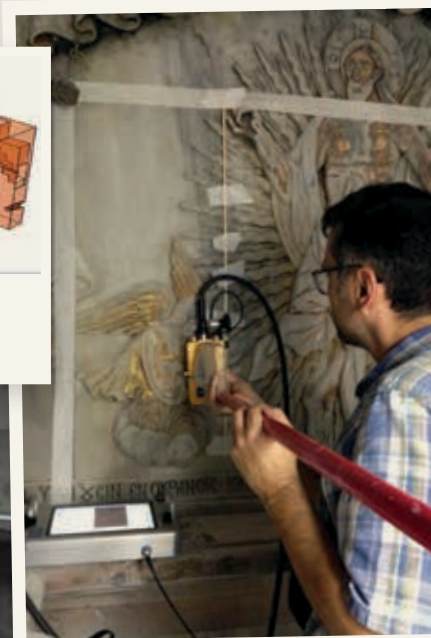
Ground penetrating radar prospecting of the Holy Aedicule of the Holy Sepulchre in order to reveal its internal structural layers
